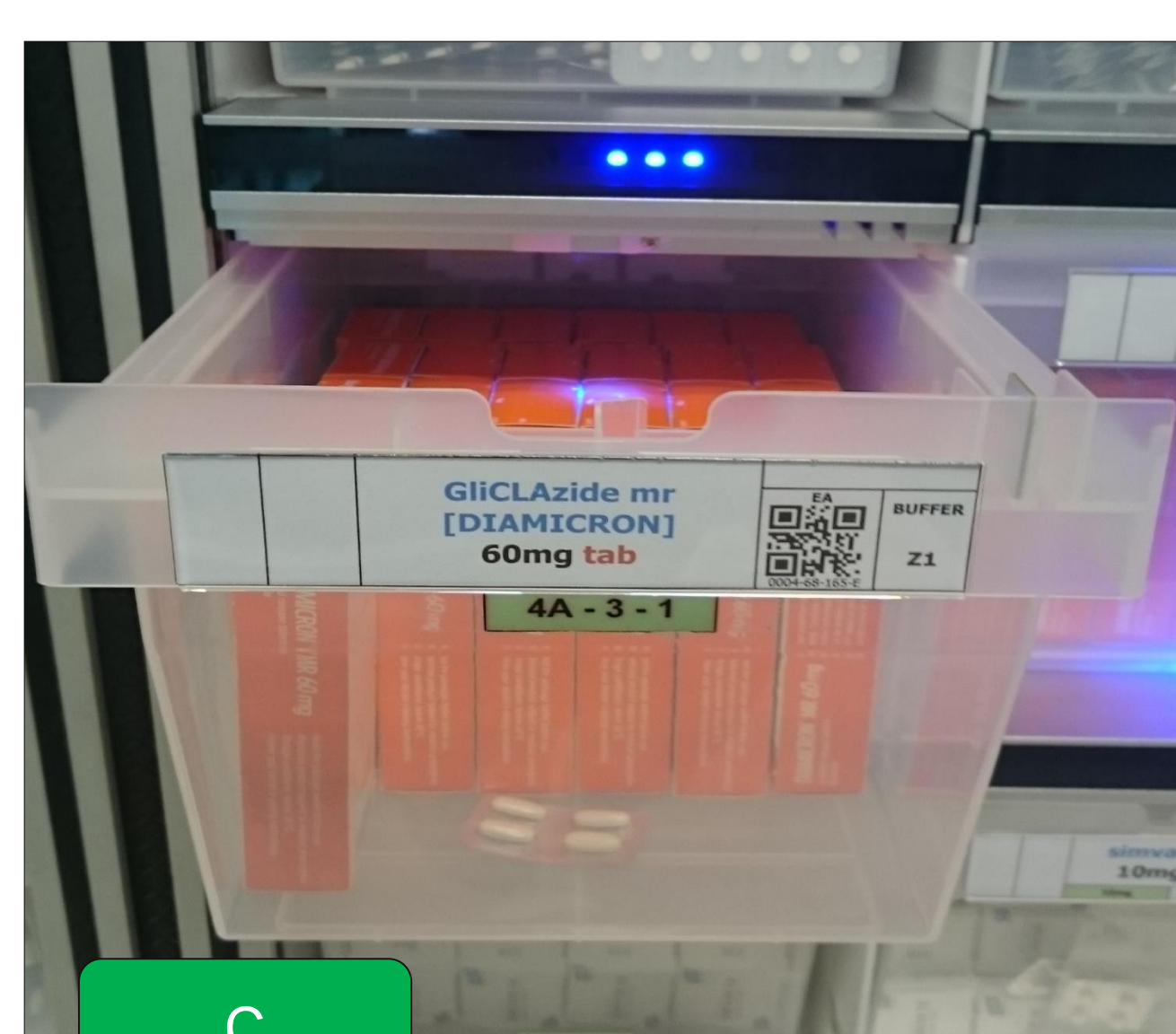
C Locking mechanism unlocks, enabling staff to pick from drug bin or to load / return drugs to drug bin
