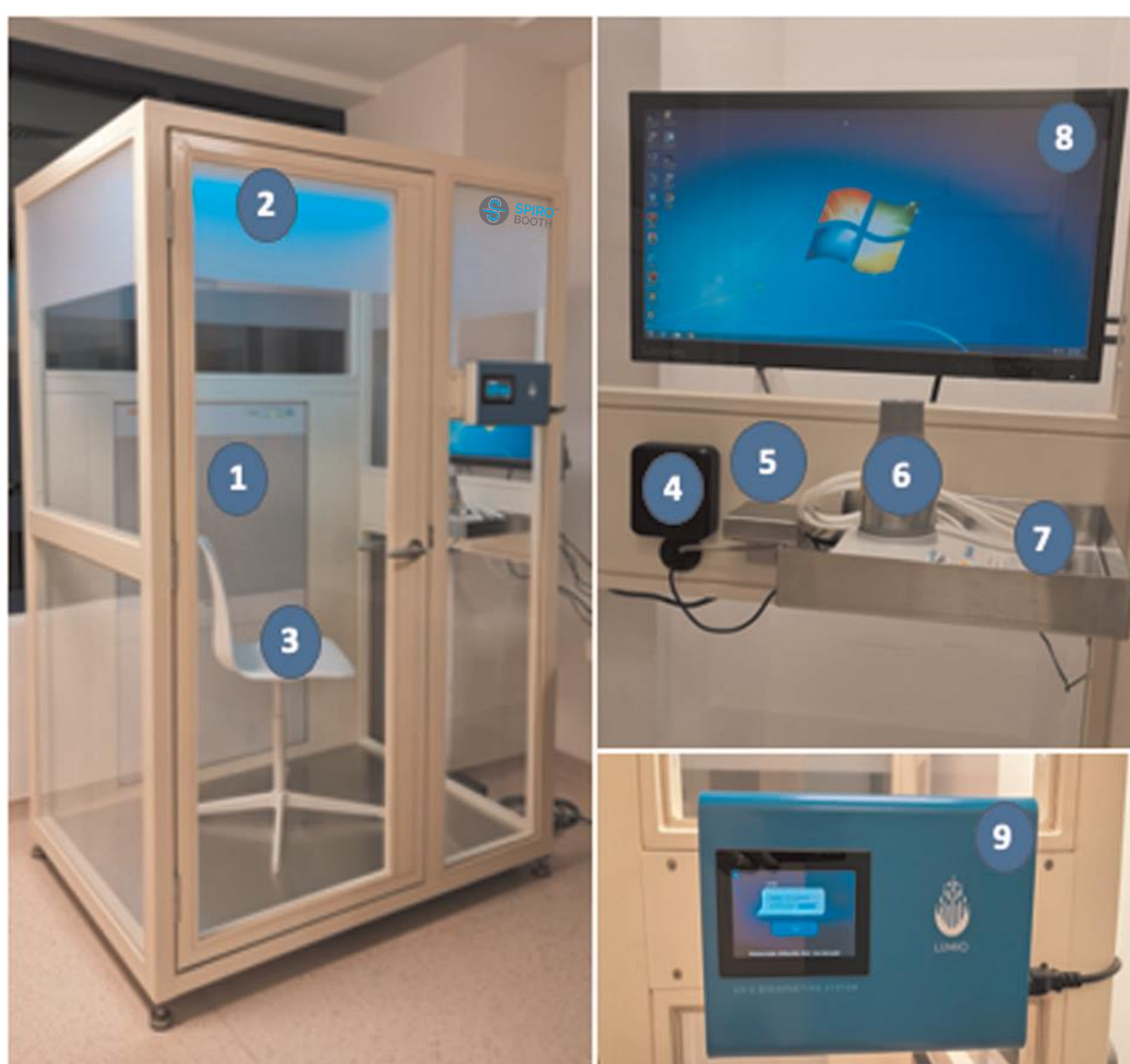
SpiroBooth. 1: AIRTECH ACP-897CH Clean Partition HEPA filter system; 2: UVC system; 3: Chair; 4: Intercom; 5: stainless steel base for the clip-on height adjustable holder for the spirometer mouthpiece (optional); 6: spirometer; 7: holder tray; 8: PC monitor; 9: UVC disinfection system control panel.
