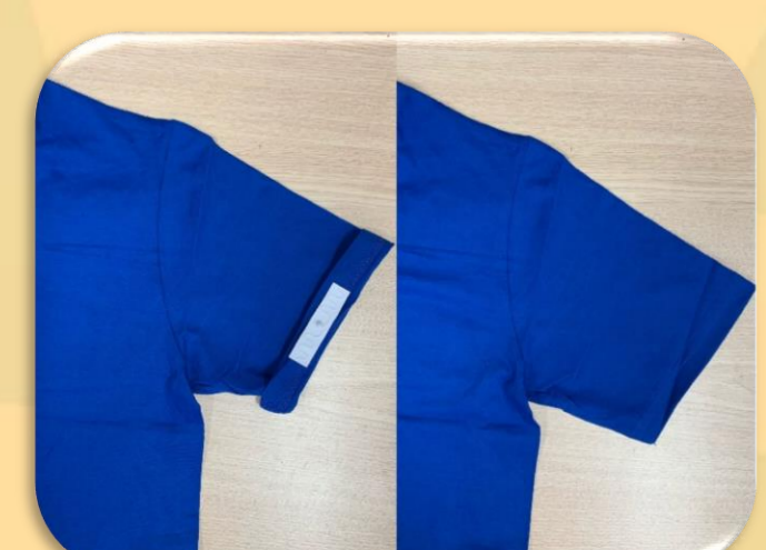
Small and water proof RFID tag/s sewn into the seams of residents' clothes
